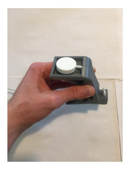
Bring the two halves together, and remove the charger cap from the watch charger.
