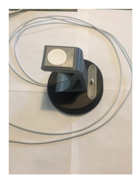
Press on the adapter piece and the watch charger cap. You may need to lightly sand the sides of the watch charger cap.
