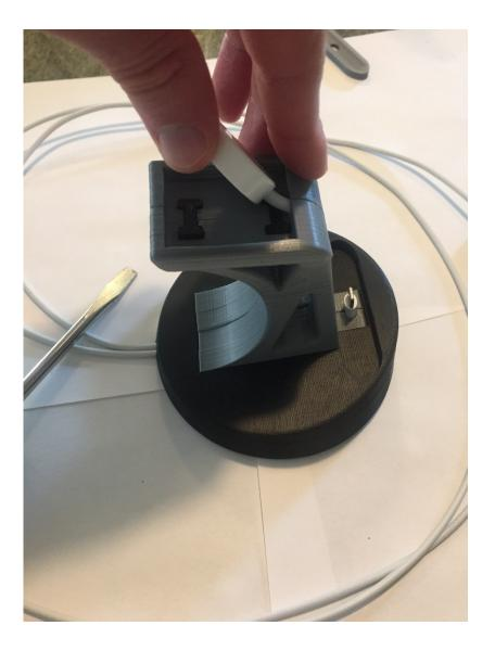
Press the two clips into the pockets under the watch charger. It helps to use a flathead screwdriver.
