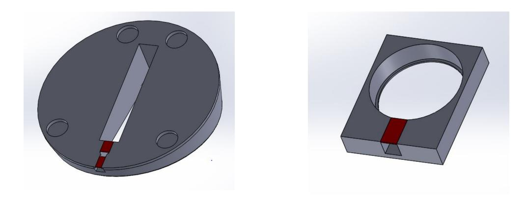
By default, the base and charger cap print with a thin connector (shown in red) to help reduce warping. Cut these prior to assembly.
