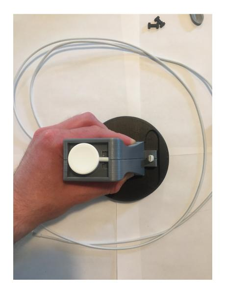
Press the two halves into the stand base. If it does not go in easily, sand the faces which are interfering.
