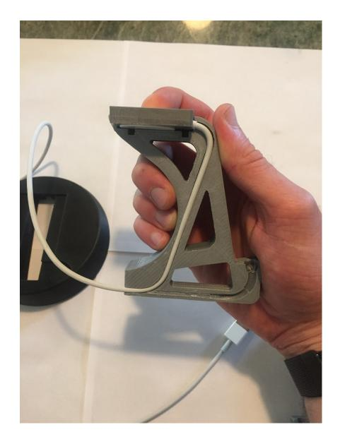
Press watch charger cap onto watch charger and lay cable in the groove.
