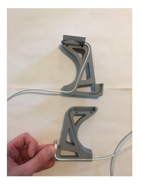
Lay the phone charging cable in the groove of the other side.
