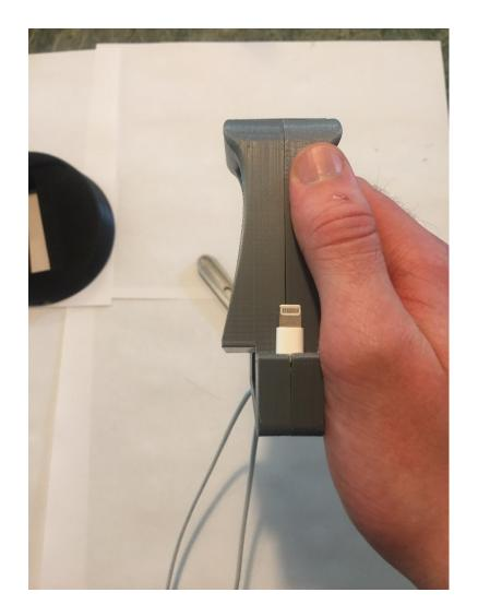
To disassemble: Remove the base, then grab one half and firmly pull down the other half while rocking it back and forth.
